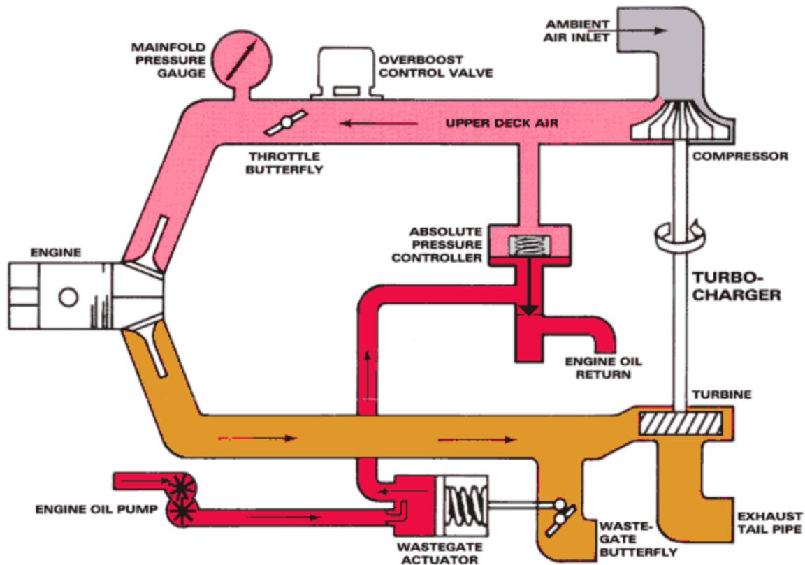
Turbocharged engines normally demand 100 octane avgas because of the high cylinder pressures. Use of lower octane fuel could lead to detonation, which is of more concern in a turbocharged engine than in a lower-compression normally aspirated engine.
